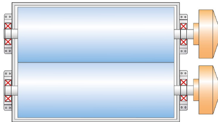
Figure 1 Principle drawing of the pulp washer.
