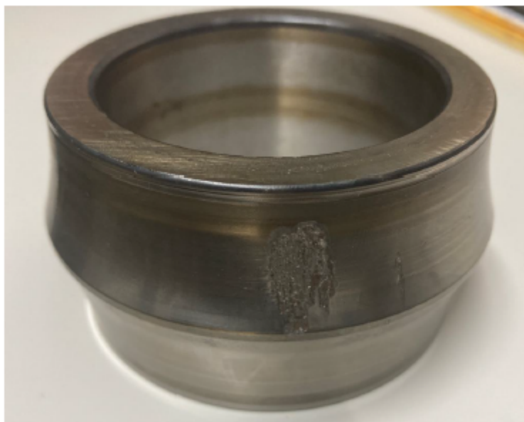
Image 5 The bearing inner race damage.
